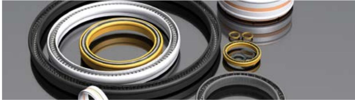
**CAAST ECup-seal** is a spring-energized U-cup jacket available in a variety of configurations for Rod, Piston, Face and Rotary applications. The sealing concept is based on the constant force applied by the internal spring that makes the external jacket resilient. As pressure is introduced in the system the seal expands increasing the initial sealing force provided by the spring.
